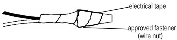
9. Connect the black fixture lead to the black wire in the outlet box. Fasten the joined wires as in step 8.
