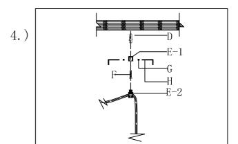
Step. 4: Install Wall anchor(D) into the ceiling, And use the tapping screw(F) to lock the wire holder cap(E-1). Then install wire holder (E-2) into cap, and use wrench(F) to tighten screw(G) to lock wire holder in the cap.
