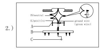
Step. 2: Wire fixture to wires in outlet box. Copper/Green wire is for Ground.
