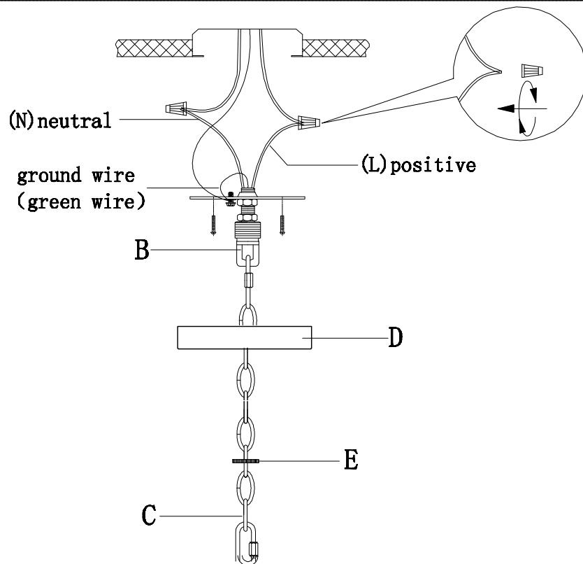
Attach appropriate amount of chain to loop to achieve desired mounting height. Thread wire through every 3rd loop of chain. Remove ring from loop and slide down chain. Place canopy onto chain and let slide to top of fixture. Install nipple and cross bar into top of chain loop.
