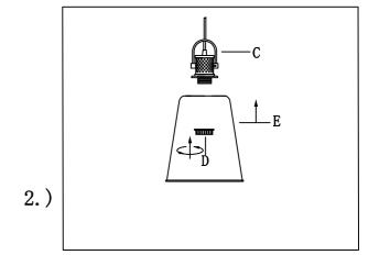
Step. 2: Use socket ring (D) to secure shade (E) on body.
