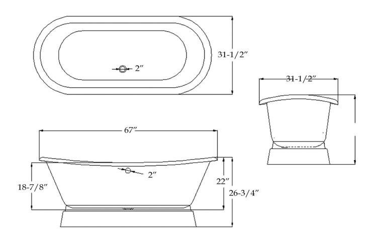
Weight (empty): 411 lbs Weight (filled): 828 lbs Capacity: 50 gal Water depth: 13"
