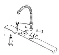
**Flushing and checking for leaks:** After the installation is complete, unscrew and remove the spray head in order to flush the line. Turn on the water supply and allow both hot and cold water to run for at least one minute each. This flushes away any debris that could cause damage to internal parts. Check for leaks. Re-attach the spray head. Do not lose the gasket (1) in the hose.
