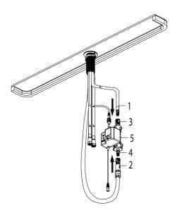
Connect the hose (1& 2) to the connector (3 & 4) on the control box (5). Push firmly together until they snap into place.
