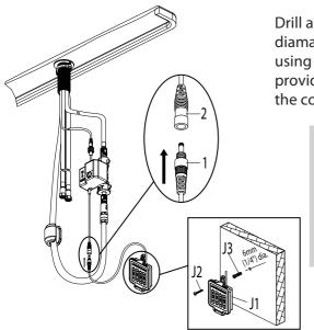
Drill a hole in the wall using a 6mm (1/4 in.) diamater drill bit. Install the battery pack (J1) using the molly anchor (J3) and screw (J2) provided. Insert the battery pack cable (1) into the control box connection (2).
