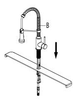
Shut off the water supply. Insert faucet body (B) through the hole inthe sink.
