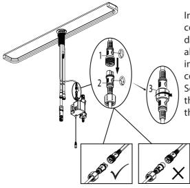
Install the data cable (1) to the control box connection (2). Ensure the arrows on the data cable and control box connection are aligned to one another to ensure proper installation. Ensure they are tightly connected by firmly pushing together. Secure the connection by hand tightening the nut (3) in a clockwise direction onto the threaded sensor cable.
