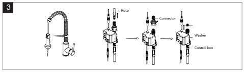
a.This could indicate that the washer in the control box is dirty or damaged. Remove the hose and unscrew the connector. Take out the washer from the control box. Clear the washer or replace the washer. Reassemble the connector and hose.
