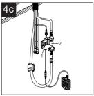
Check whether the switch button (1) is tighten, if it is loose, tight the switch button (1) completely with a coin clockwise. If the switch button (1) is tighten, this indicates that the control box (2) is damaged. Call customer service to request a replacement control box. Replace the old control box with the new control box.
