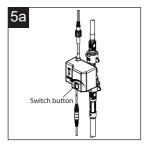
If you want to use the faucet without the sensor feature, you can loose the switch button completely with a coin counterclockwise. At this time, you can use the sensor faucet as the use of the common faucet.
