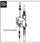
However, if you want to continue to use the faucet with the sensor feature, you need tight the switch button completely with a coin clockwise. At this time, you can use the faucet with the sensor feature.
