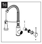
This indicates that the cartridge is damaged. Turn off the water supply, remove the handle and replace the cartridge (1).
