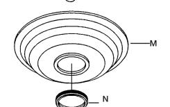
1) Screw loop onto threaded pipe on top of fixture.
