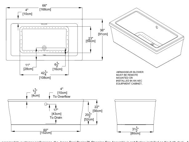
NOTE: To accommodate customer preferences, the Jason Sani-Design™ Cleaning Cap Assembly is not factory installed on the bath deck. An Installation Kit for the Sani-Design™ Cleaning Cap is provided with this bath.
