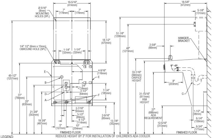
A = Recommended Water Supply location. Shut-off Valve (not furnished) to accept 3/8" O.D. unplated copper tube. Up to 3" (76mm) maximum out from wall. B = Recommended Waste Outlet location. To accommodate 1-1/4" nominal drain. Drain stub 2" (51mm) out from wall.
