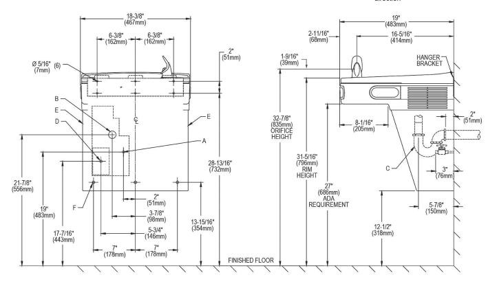
A = Recommended water supply location. Shut off valve (not furnished) to accept 3/8" O.D. unplated copper tube connect. Up to 3" (76mm) maximum out from wall. B = Recommended waste outlet location. To accomodate 1-1/4" nominal drain. Drain stub 2" (51mm) out form wall.
