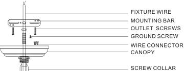
All electrical components must be installed by a licensed electrician in accordance with the National Electric Code and the appropriate local electrical codes.
