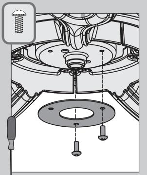
Align the screw holes in the switch
