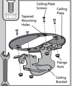
Align the tapered mounting holes in the ceiling plate with the holes in the ceiling bracket. Install the four ceiling plate screws found in the hardware bag and secure with the flange nuts using an 11/32" wrench. Hold the ceiling bracket assembly up to the outlet box and mark the screw locations. To mount to support structure, also mark the ceiling for drilling pilot holes.
