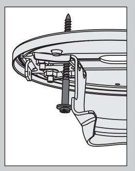
Use the wood screw to poke holes through the rubber gasket in order to install the ceiling bracket assembly to your support structure or ceiling fan-rated outlet box. Use wood screws (included) and washers when securing to support structure with approved electrical outlet box. Drill 9/64" pilot holes in support structure to aid in securing ceiling bracket with hardware found in the ★ hardware bag.
