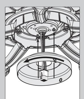
Feed the 9-pin connector plug through the center hole of the upper switch housing, then wrap keyhole slots around the screws and twist counterclockwise.
