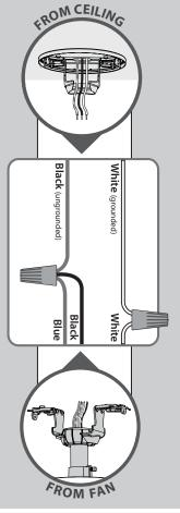
Using orange wire connectors from the  $\bigstar$  hardware bag, connect the black wire (ungrounded) from the ceiling to the black and the blue wires from the fan. Connect the white wire (grounded) from the ceiling to the white wire from the fan.
