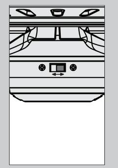
To switch the direction of air flow, move the reverse switch to the opposite position.
