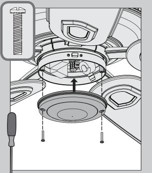
Lift the lower switch housing up until the holes line up with the screw holes in the upper switch housing. Install the two switch housing screws, found in the = hardware bag.
