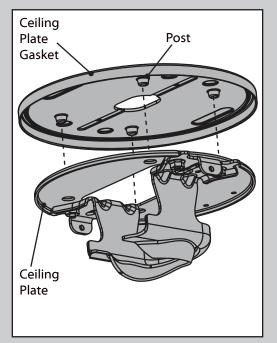
Install the ceiling plate gasket onto the ceiling plate. The four holes in the ceiling plate should lineup with the four posts in the gasket.
