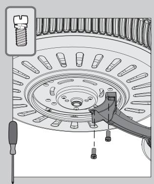
Lightly attach the blade irons to the motor with screws found in the X hardware bag, then securely tighten after both screws are attached.
