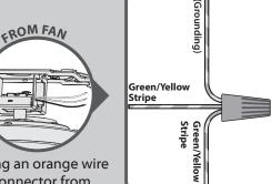
Using an orange wire connector from the \* hardware bag, connect the 3 grounding wires (green, green/yellow stripe, or bare copper) coming from the ceiling, fan, and hanging bracket.
