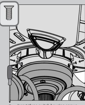
Insert three switch housing screws found in the  $\equiv$  hardware bag.
