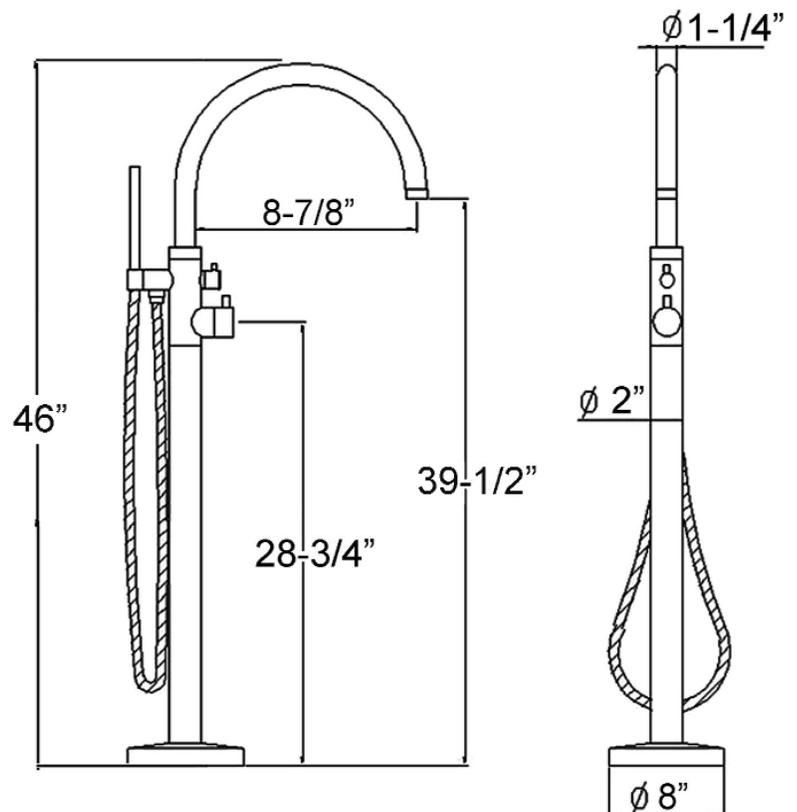
**Use on concrete floors requires special installation. We recommend using a plumbing professional.**
